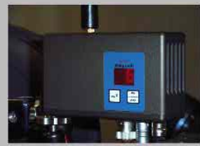
single transmitter 80 mW auto record signal and line out 95mm W x 60mm L x 35mm
